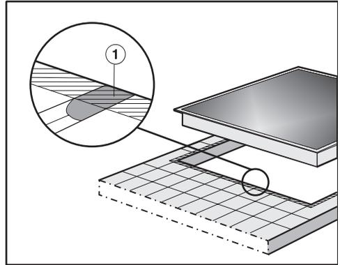
The grouting ① and the hatched area below the cooktop frame must be smooth and flat, so that the frame will be level and the sealing strip under the edge of the upper part of the cooktop can provide an adequate seal against the countertop.
